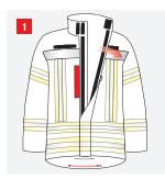
The Rosenbauer IRS belt is inserted through an internal tunnel in the jacket.
