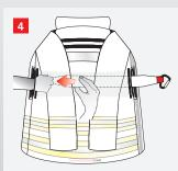
The belt is fully inserted and the two loops that can be attached to a carabiner.
